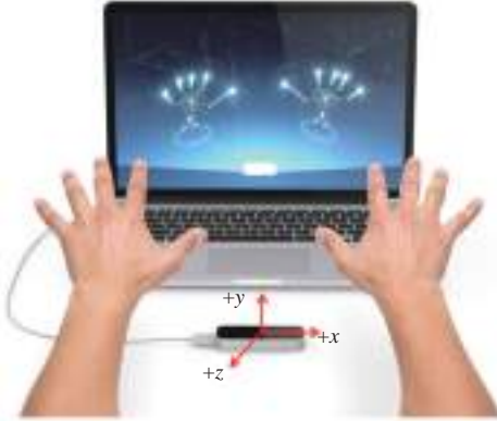
Fig. 5. The coordinate system of the Leap Motion.
