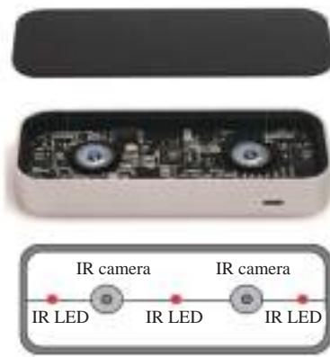
Fig. 2. The structure of the Leap Motion.
